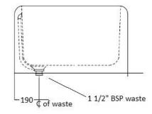
Waste and overflow fitting finishes 50mm into the floor
