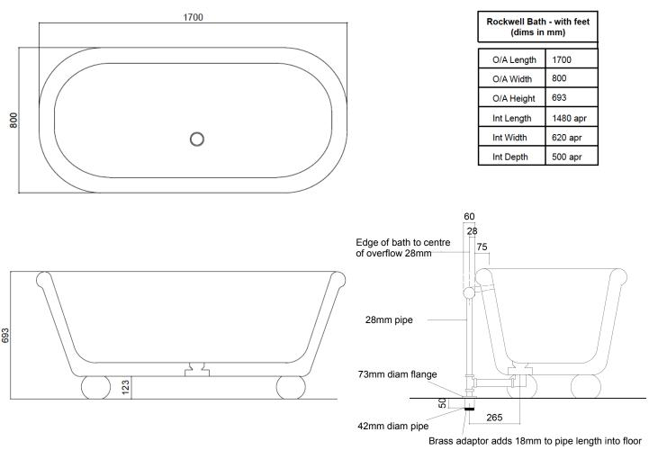
Waste: 1 1/2"; Overflow: 28mm into 42mm waste pipe - outlet is 1 1/2" BSP. We only supply fittings above the floor. We do not supply the trap; the trap needs to go beneath the floor. Dimensions are given in mm, they are a guide only and may vary from bath to bath.
