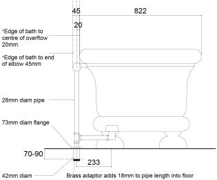
Waste: 1 1/2"; Overflow: 28mm into 42mm waste pipe - outlet is 1 1/2" BSP.
