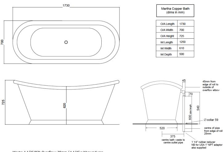
Waste:  $1 \frac{1}{2}$  BSP; Overflow: 28mm /  $1 \frac{1}{4}$  rubber reducer. We only supply fittings above the floor. We do not supply the trap; the trap needs to go beneath the floor. Dimensions are given in mm, they are a guide only and may vary from bath to bath.
