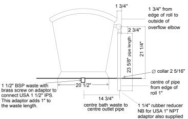
Waste: 1 1/2" BSP // 1 1/2" IPS; Overflow: 28mm / 1 1/4" rubber reducer.
