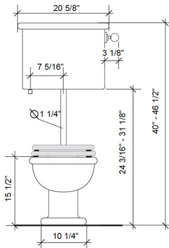
Cistern inlet pipe position diagram
