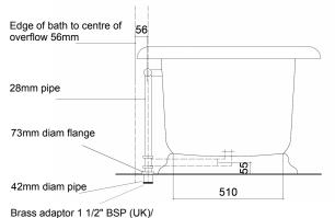
The outlet pipe can be used horizontally by turning the 'T' and can be supplied with an extra pipe and elbow if wishing to go into the floor further behind the bath if specified.
