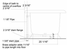
The outlet pipe can be used horizontally by turning the 'T' and can be supplied with an extra pipe and elbow if wishing to go into the floor further behind the bath if specified.
