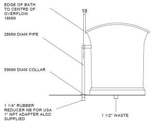
Waste: 1 1/2" BSP; Overflow: 28mm / 1 1/4" rubber reducer.
