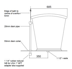
Waste: 1 1/2" BSP; Overflow: 28mm / 1 1/4" rubber reducer.
