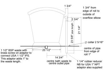
Waste: 1 1/2" BSP // 1 1/2" IPS; Overflow: 28mm / 1 1/4" rubber reducer.
