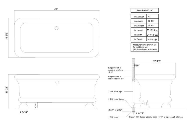
Waste:  $1 \frac{1}{2}$ ; Overflow: 28mm into 42mm waste pipe - outlet is UK  $1 \frac{1}{2}$  BSP - USA  $1 \frac{1}{2}$  IPS. We only supply fittings above the floor. We do not supply the trap; the trap needs to go beneath the floor. Dimensions are given in inches; they are a guide only and may vary from bath to bath.
