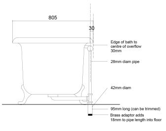
The outlet pipe can be used horizontally by turning the 'T' and can be supplied with an extra pipe and elbow if wishing to go into the floor further behind the bath if specified.
