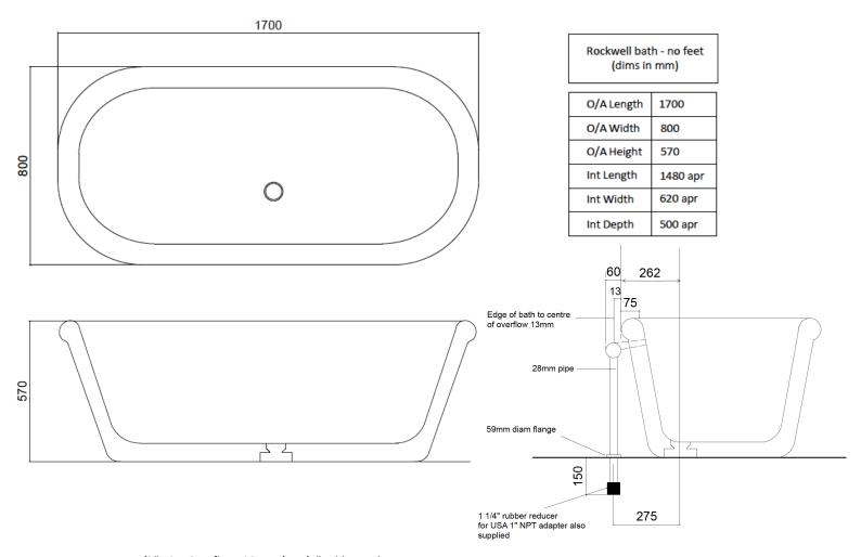
Waste: 1 1/2" BSP; Overflow: 28mm / 1 1/4" rubber reducer.
