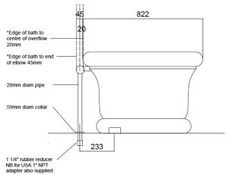
Waste: 1 1/2" BSP; Overflow: 28mm / 1 1/4" rubber reducer.
