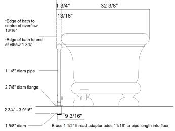
Waste:  $1\,1/2$ "; Overflow: 28mm into 42mm waste pipe - outlet is UK  $1\,1/2$ " BSP - USA  $1\,1/2$ " IPS. We only supply fittings above the floor. We do not supply the trap; the trap needs to go beneath the floor. Dimensions are given in inches; they are a guide only and may vary from bath to bath.
