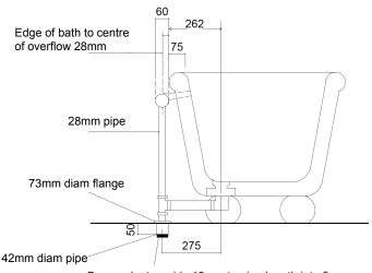
Brass adaptor adds 18mm to pipe length into floor
