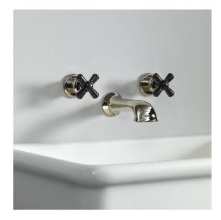
**Technical Details** Valve rough-in depth maximum: 95mm Valve rough-in depth minimum: 50mm Primary material: brass Valve fittings hole diameter: 30mm Spout fittings hole diameter: 25mm Handle turn angle: 1/4 turn Spout length: 165mm Spout inlet connection size: 1/2" BSP Spout inlet connection type: male Inlet connection size: 1/2" BSP Valve inlet connection type: female Installation type: wall mounted Number of handles: 2 Number of holes: 3 Spout swivel: no Suggested application: basin
