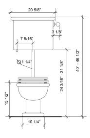
Cistern inlet pipe position diagram
